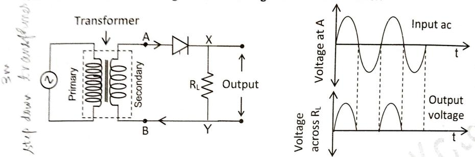
The secondary of a transformer supplies the desired ac voltage across terminals A and B. When the voltage at A is positive, the diode is forward biased and it conducts. When A is negative, the diode is reverse biased and it does not conduct. Thus the current flows through the circuit during positive half cycles. The current through  $R_L$  is from X to Y, unidirectional. Thus output voltage is unidirectional as shown in the graph.
