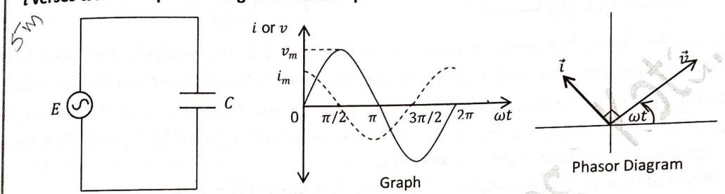
Consider a capacitor of capacitance C, connected across an A. C. source. Let the voltage across the source be  $v=v_m\sin\omega t$ . Let q be the charge on the capacitor at any time t.
