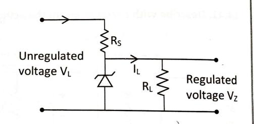
Similarly if the input voltage decreases, the current through  $R_S$  and zener diode also decreases. The voltage drop across  $R_S$  decreases without any change in the voltage across zener diode.
